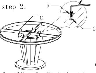
Connect Table top frame(C) to Stainless steel pillar (B) with bolts (F) (M8\*30), Tighten
