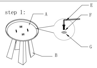
Connect Stainless steel pillar (B) with Stainless steel base (A) by Screw (F) (M8\*30), tighter, one by one
